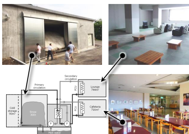
Figure 3. Snow-cooling system for a spa resort.
