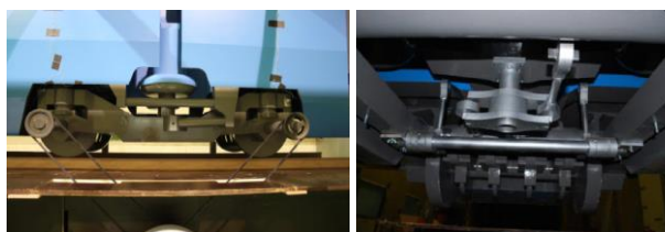
Figure 17: TGV bogie model including anti-roll bar and the bogie-car drive system
