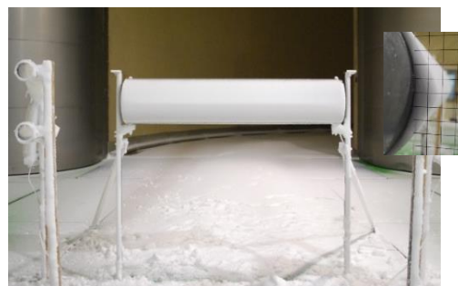
Figure 19. Experimental and numerical modeling of wet snow impact and accretion cylinders of various diameters (diam. 50, 200 and 315mm)
