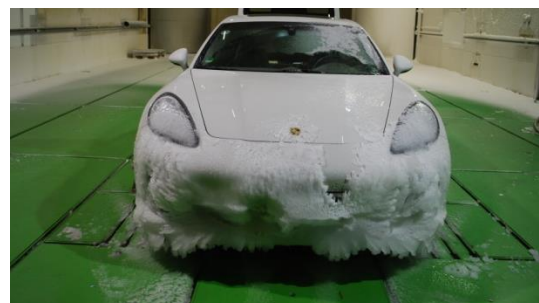
Figure 6. Wet snow accretion on the front panel of a road vehicle
