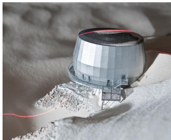
Figure 18. Small-scale model in the wind tunnel (H. Raguet)
