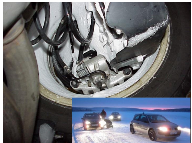
Figure 11. Snow braking test on a frozen lake in Kiruna
