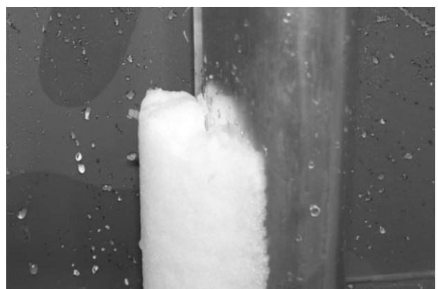
Figure 5. Example of wet snow accumulation (after partial shedding) on a mullion in a climatic chamber simulation.
