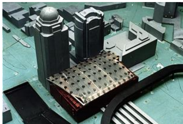
Figure 4. Measurement of surface wind velocities in an RWDI wind tunnel for FAE method
