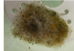
Initial contamination of a new bio-based insulation material by *Trichoderma*.
