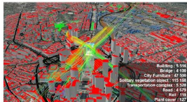
Figure 1. Partial view of the generated BIM model in CityGML format including CFD simulation results.
