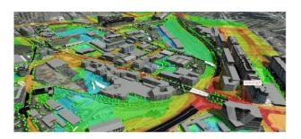
Figure 9. Integration of a horizontal noise map exported from MithraSIG as a SHP file into the BIM model.
