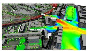
Figure 15: Pedestrian wind comfort map inserted in the BIM model
