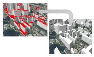
Figure 4. Application of the CityGML LOD2 to LOD1 transformation algorithm to buildings objects.
