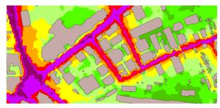
Figure 6: Generated Lden horizontal noise map. dB values vary between below 45 (deep green) to above 75 (deep purple).
