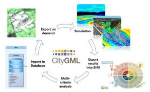
Figure 2. Schematic of the BIM simulation integrated process
