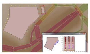
Figure 7: Example of building facade noise level calculation (same color code as above)
