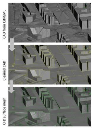
Figure 12. Illustration of the process to generate a correct CFD mesh from the CityGML model
