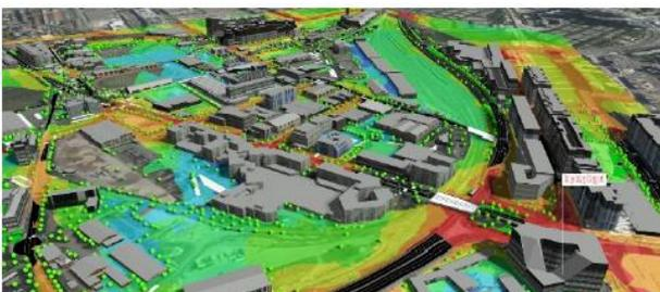
Figure 9. Integration of a horizontal noise map exported from MithraSIG as a SHP file into the BIM model.
