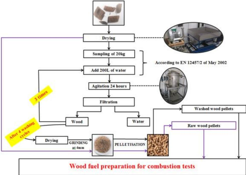
Fig. 1. Wood fuel preparation for combustion tests.
