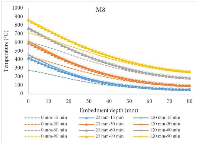
Fig. 7: Temperature profiles for M8 and M12 anchors with  $h_{ef}=10*d$  for different extended lengths
