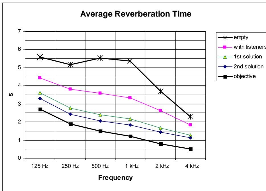
Figure 4.- Reverberation time of different proposed solutions for the chapel
