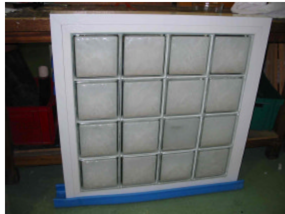
Figure 2: Glass bricks wall containing PCM
